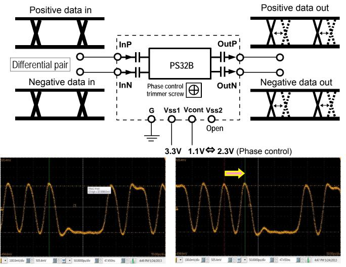
32-Gb/s pattern triggered waveforms when voltage of Vcont was set to 1.1 V (left) and 2.3 V (right). 62.5-ps time delay was obtained.
